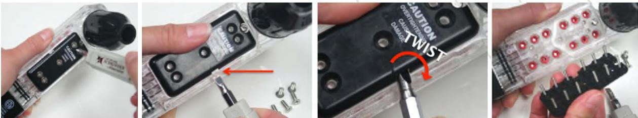
Use the O-ring Insertion and Extraction Tool to remove the plunger assemblies and the black O-rings. These parts may need to be removed separately. Use the barbed end of the tool when removing the components.
