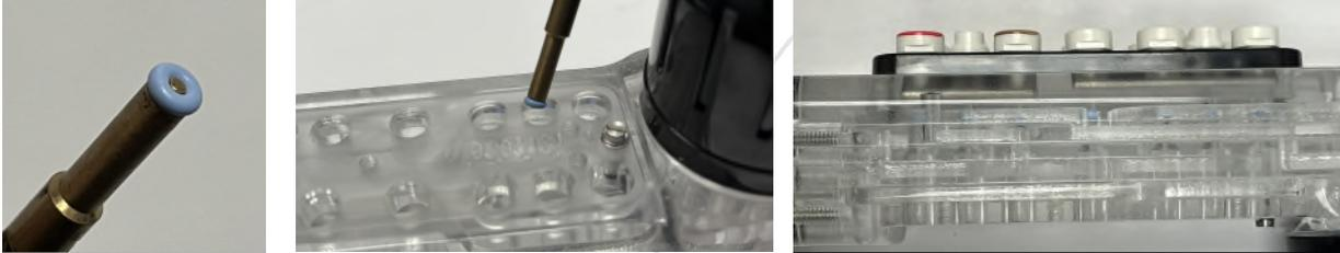
Reinstall the plunger assemblies and the bottom plate, taking care not to bend the plunger springs. Use the screwdriver to resecure the plate without overtightening.
