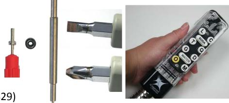
Use the Phillips head screw driver to unscrew the 5 Phillips head screws on the bottom plate of the handle and place aside
